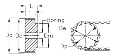
Belt width Type = T10= - 25 mm Weight = 1.31= 138.2De Dm = 88 = 140.2Dp F = 30 L = 40 Pre-drilled = 10 Tooth number = 44
